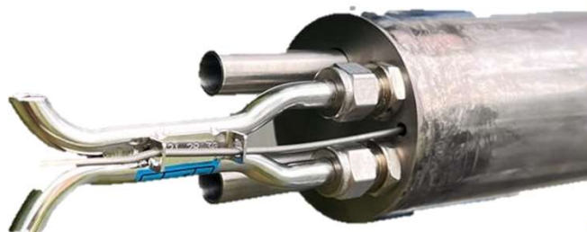
Sampling probe with Pitot tube and sampling tubes
